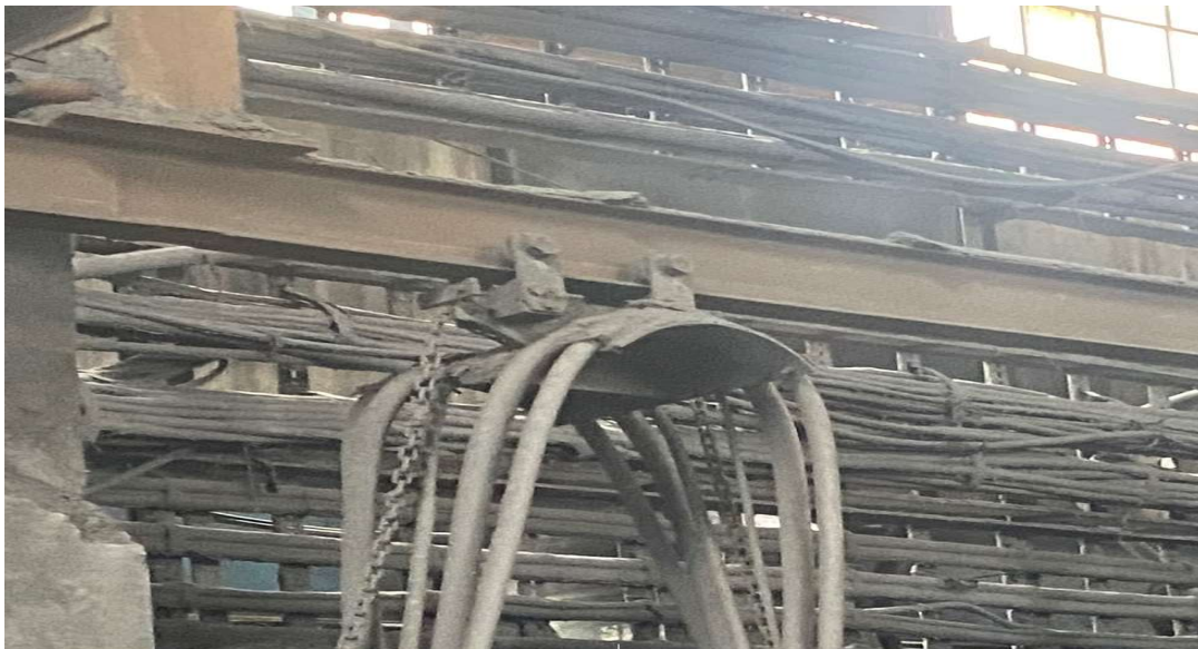
Existing Festoon Trolley guide roller/channel /chain arrangement
