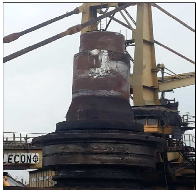
Damaged shaft matching with hollow shaft
